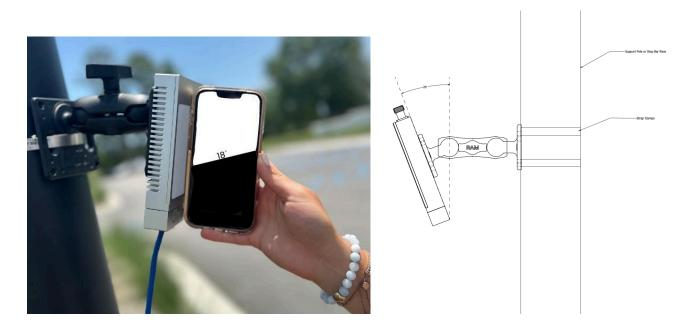
• Ensure Horizontal Level: Confirm that the sensor is horizontally (verify if vertically) level and securely fastened to the mounting bracket.
