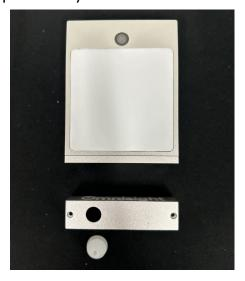
• After pushing the Cat 6 wiring through the rubber grommet insert the wiring through the opening in the lower housing unit.
