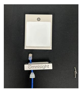
• Insert the RJ45 Jack into the RJ45 network port on the upper portion of the Fusion Sensor.
