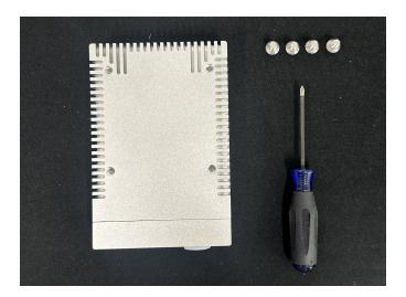
Position one of the ram ball mount brackets over the back side of the fusion sensor and use the phillips head screwdriver to attach the mount bracket to the rear of the Fusion Sensor.
